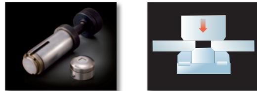
Reduce costly and time-consuming, post-punch deburring by doing the work "in the sheet." Use of the deburring tool ensures that burrs raised during the punching process are flattened – resulting in improved edge quality while streamlining the manufacturing process.
