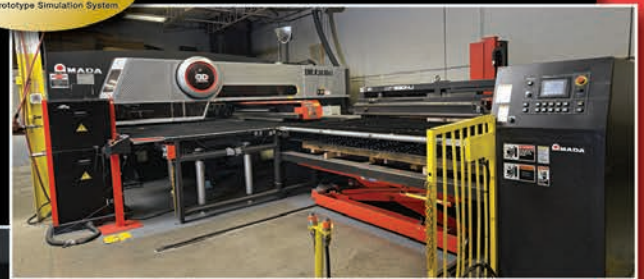
EMLK punch/laser combination with MP automated load/unload system.
