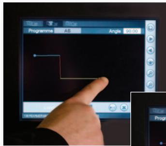
Drawings can be made directly into the NC by using the new touch-screen technology.
