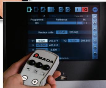
For special applications, manual mode programming allows the operator to create personalized programs.
