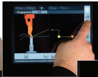
The NC control is capable of generating programs automatically. It takes into account bending constraints and ergonomics, including gauging position, component handling, bend order and required tolerance.
