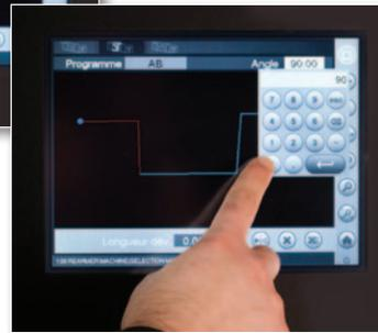
The operator enters the dimensions into a pop-up window. It is also possible to indicate bending priority.
