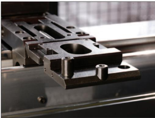
A Delta-X option is also available for the rear backstop of the 7-axis machine. This provides the stop fingers with an additional incremental adjustment of  $\pm 6''$  in the X-direction. Both stop fingers can be set to different depth measurements – particularly helpful in the case of asymmetrical workpieces. Available as a single option or as a pair.
