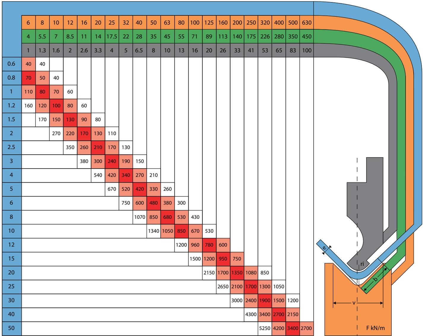
This example of an air-bending force chart is for mild-steel (40-45k/mm<sup>2</sup> tensile strength). From the material thickness it is possible to determine:
