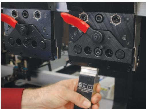
Amada's S-GRIP punch holder allows the brake operator to change punches on the press brake quickly and safely without requiring a wrench. The patented S-GRIP design dramatically decreases tool changeover time, thereby increasing bending productivity
