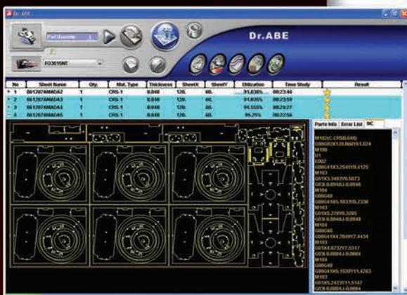
Dr.Abe\_Blank software automatically creates nesting data with unmatched speed and ease of use — enabling Cyrell to successfully support high-mix, low-volume production.
